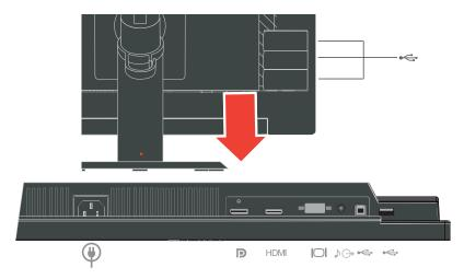
3. Connect one end of the DP cable to the DP connector on the back of the computer, and the other end to the DP connector on the monitor. Lenovo recommends that customers who require to use the Display Port input on their monitor purchase the "Lenovo Display Port to Display Port cable 0A36537".
